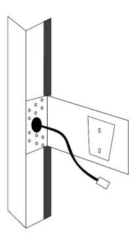
The window mount is now ready for the Concierge Room Booking Display to be mounted. Slide on the display, connect the required cables and screw on the 2 x M5 screws provided with a hand held screw driver. The screw points are located at the base of the bracket.
